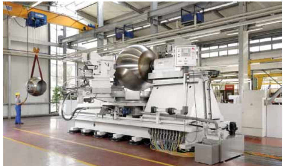
Picture 1: KDSM 1400 for balls with outer diameter 1.200 – 2.010 mm.
