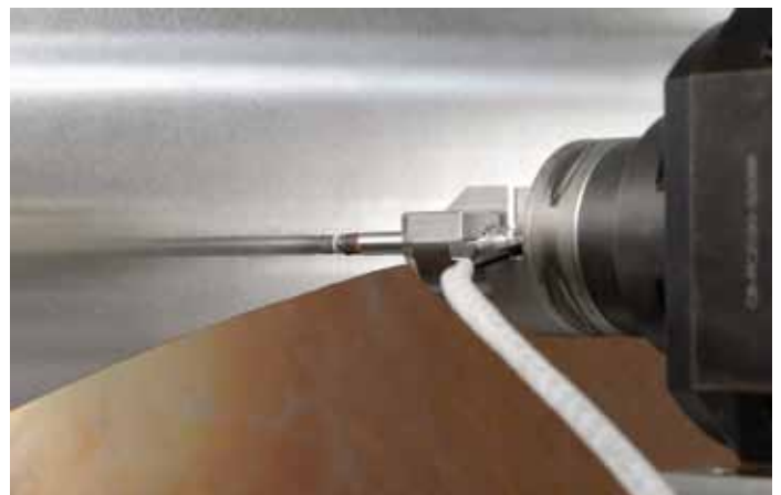
Picture 3: Integrated measuring of shape tolerance and outer diameter.
