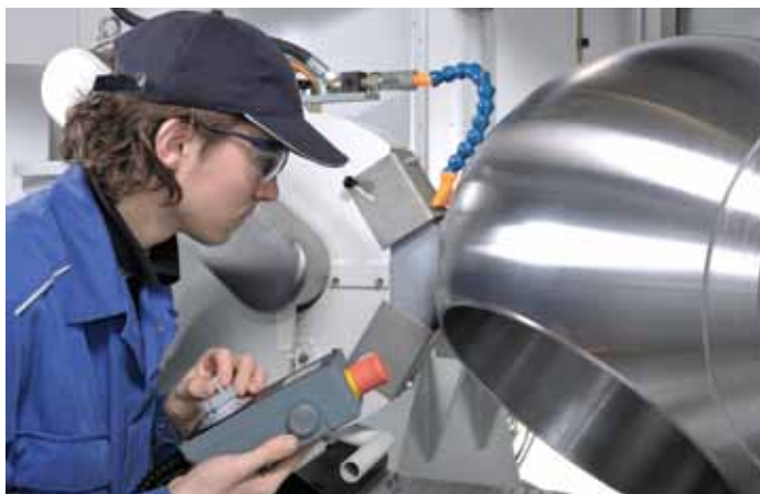
Picture 2: Locality variable panel for manual operation and setup.
